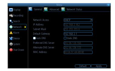
**Network Access:** Here you can choose between the three different types of networks that the DVR can be connected to. The three types of networks are:
