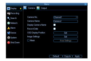
**Camera No.**: Choose the camera / channel you want to edit here. The Camera No is the same thing as the number written on the rear panel next to the BNC socket used to connect the camera.
