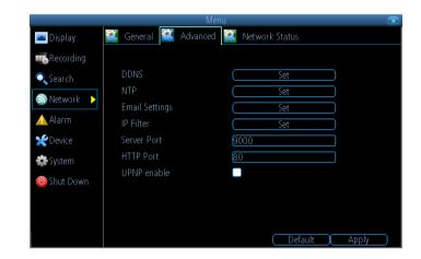
**DDNS:** The place to configure the DVR to automatically update a dynamic DNS service. If you want to remotely access the DVR via the Internet, you'll probably need to configure a DDNS account. See "Network: Advanced: DDNS" for details on setting up and configuring the DDNS.
