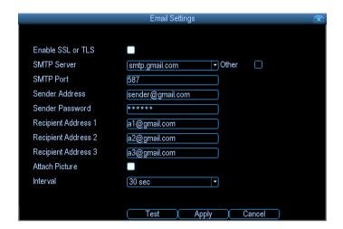
**Enable SSL or TSL:** Whether the email server you're using requires a secure link. This is on be default, and should be left on if you're using any of the preset email servers.
