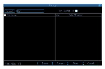
**Refresh:** Looks for devices to which footage can be backed up. This will include USB flash drives or hard drives connected to the USB port, or external hard drives connected via the rear eSATA port.
