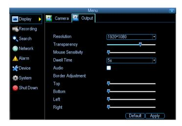
**Resolution:** Resolution should be set as high as possible, but equal to or lower than the maximum resolution your screen/monitor can display. Things change a little depending on what kind of monitor you're using, and how it's connected.
