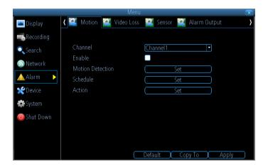
**Channel:** Which channel/camera you'd like to set the Video Loss behavior for.**Enable:** Whether or not motion detection is enabled on a specific channel. Each channel can be configured independently of one another.
