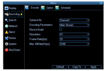
**Camera No.:** The camera feed you want to alter the settings for. These will be numbered sequentially, and correspond to the BNC video inputs labeled on the rear of the DVR. Note that the channel name here is independent of the Camera Name selected on the Display: Camera menu screen.
